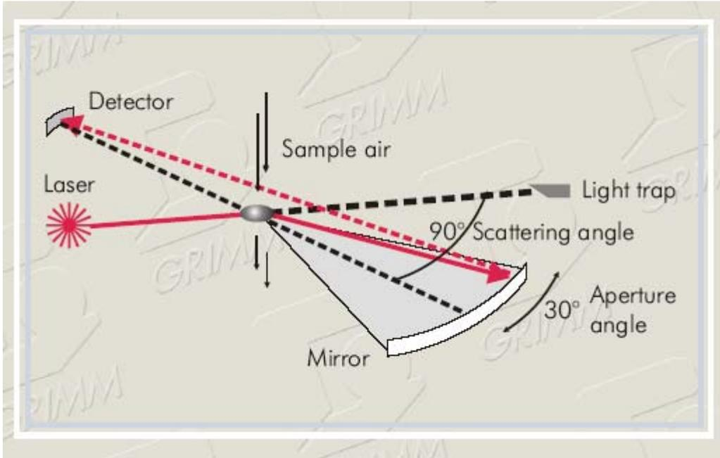
Figure 1 – Grimm detector principle
