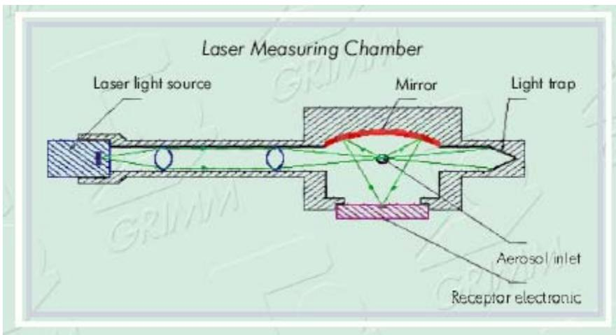
Figure 2 – Grimm Measurement Chamber
