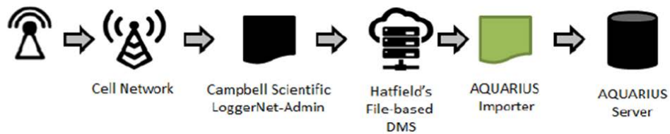
Figure 3 The process for acquiring data describing water quality, benthic invertebrate communities, snow depth, sediment quality and fish populations from field sample collections and laboratories.
