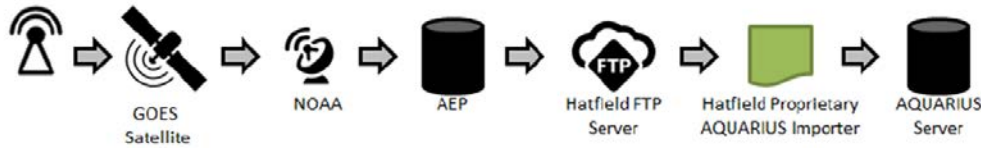
Figure 2 The process for acquiring data from climate, hydrology, and datasonde stations with cell-modem based telemetry.
