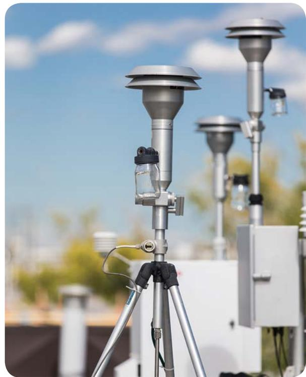
Figure 1: Instruments to monitor and collect particulate matter data used in CAAQS and AQHI reporting.
