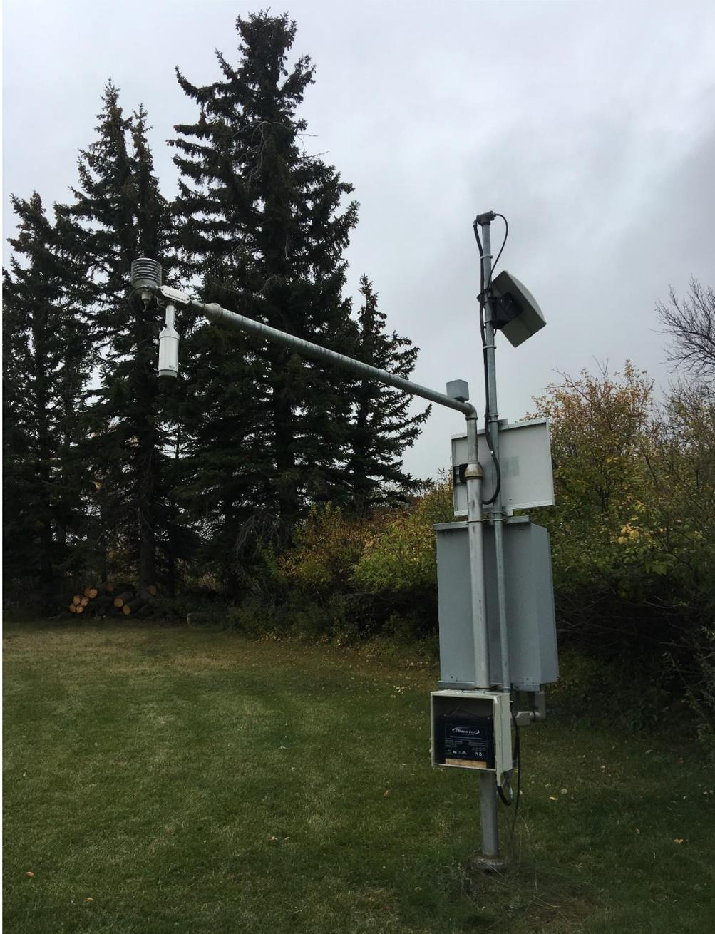
**Figure 1.** Sample Photo of a Completed Snow Depth Sensor Installation of the SR50A/SR50AT Sonic Ranging Sensor
