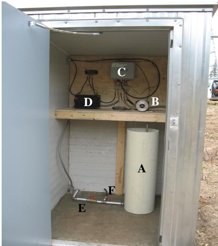
**Figure 2.** Inside of Instrument Shelter for Snow Pillow: (A) Standpipe (B) Shaft Encoder (C) Data Collection Platform (D) 12-Volt Wet Cell Batteries (E) Main Line Connected to Snow Pillow (F) Sampling Valve for Specific Gravity.
