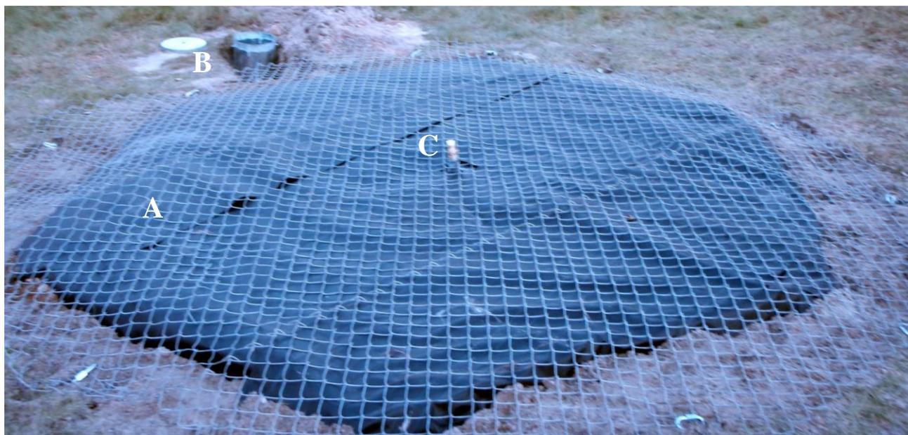
**Figure 1.** Sample Photo of a Completed Snow Pillow Installation: (A) Snow Pillow Covered by Prison Grade Chain Link (B) Shut-Off Valve (C) Two-Way Ball Valve.
