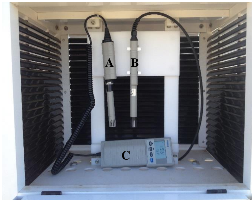
Figure 1. Inside of Stevenson Screen: (A) Standard Probe (B) Station Sensor (C) Standard Display.
