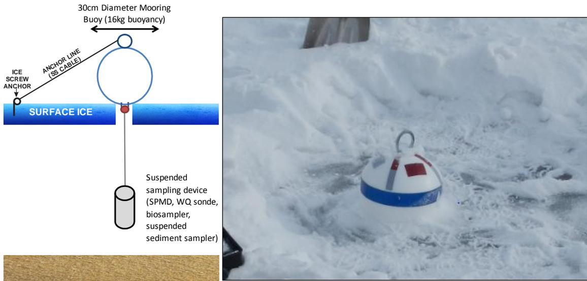
Figure 2. Suspended under-ice design.
