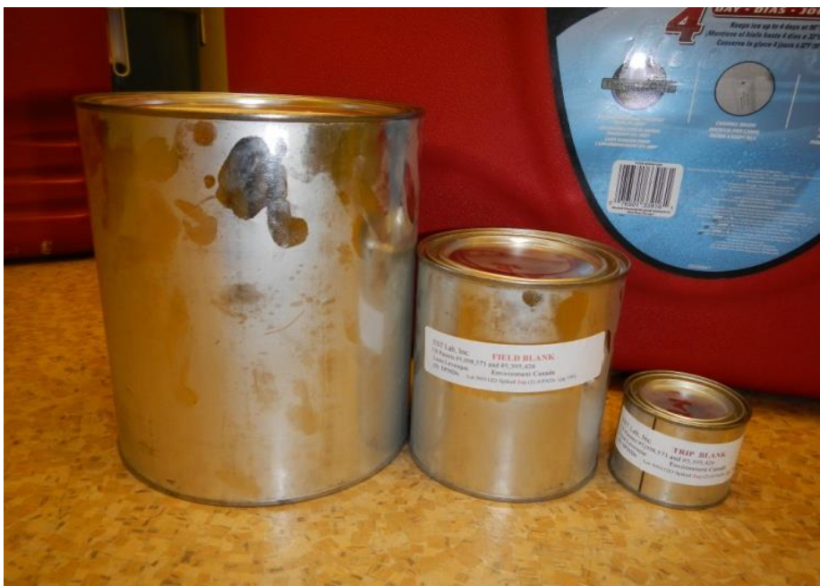
Figure 2. Semi-permeable membrane device tins. The large tin is representative of a sample membrane, the medium tin represents a field blank, and the small tin represents travel/dialysis/spike blanks.
