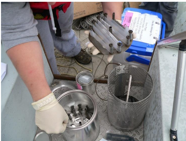
Figure 1. Preparing for the field deployment of a membrane and spider (top right) and canister (bottom right).
