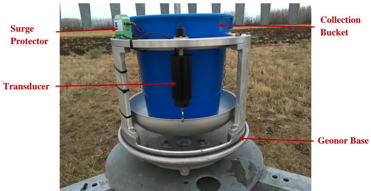
**Figure 1.** The Geonor T-200B Series Precipitation Gauge.
