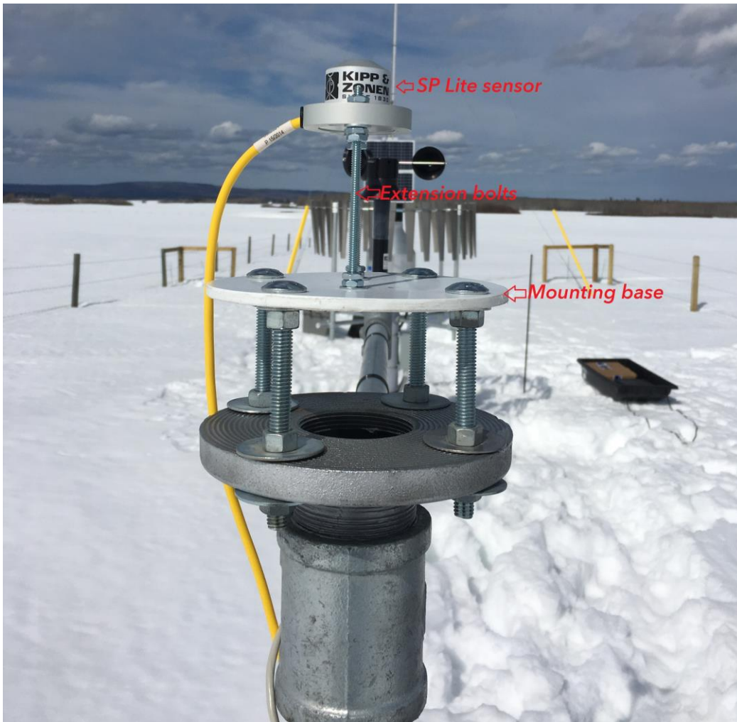
Figure 1. SP Lite Incoming Solar Radiation Sensor Installed on Extended Platform.
